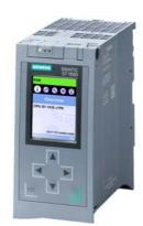
\*\*\* Spare part \*\*\* SIMATIC S7-1500, CPU 1515-2 PN, central processing unit with work memory 500 KB for program and 3 MB for data, 1st interface: PROFINET IRT with 2-port switch, 2nd interface: PROFINET RT, 30 ns bit performance, SIMATIC Memory Card required
